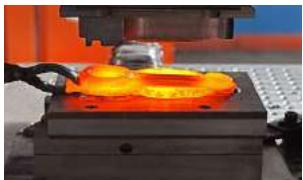
BMY products are manufactured with hot forging method.
